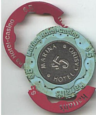
Above is a scan of the inside core of a \$5 Harrah's metal insert chip with the outer shell peeled away that should help to illustrate how these chips are constructed and why the “mini-i” variation is indeed a legitimate chip variation from a different mold.
