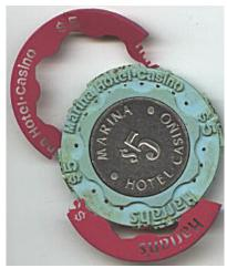
Above is a scan of the inside core of a \$5 Harrah's metal insert chip with the outer shell peeled away that should help to illustrate how these chips are constructed and why the "mini-i" variation is indeed a legitimate chip variation from a different mold.
